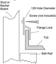
Holds tub or shower pans against wall while allowing environmental expansion and contractions without cracking the tub or shower pan. Stainless steel to prevent rusting or discoloration while providing a strong "spring" action.
