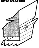
Fills gap between door and door bottom to prevent air, dust and water entry. Additional seal at the top, to stop water seepage. Pre-punched slotted holes. Includes self tapping screws. 36" long.
