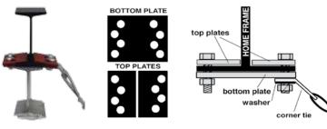
Use outside holes for 3-1/2" to 4" flanges; use inside holes for 2" to 3" flanges. For Wind Zone 1. 4 1/2" x 1-1/2" Grade 5 machine bolts and 8 1/2" high strength washers included.
