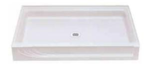
Beveled inside perimeter lets water from the walls flow back into pan. New design also adds strength. 32" x 32".
