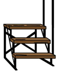
Two steps with the third step being a 19" x 29" half platform with rail for safety.
